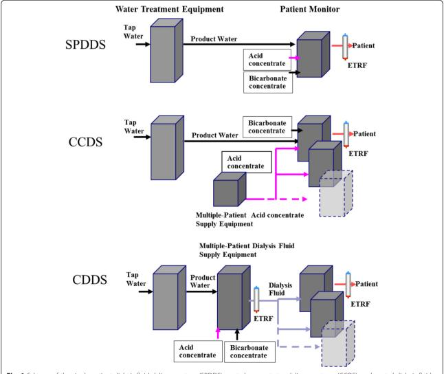
Fig. 1 Scheme of the single-patient dialysis fluid delivery system (SPDDS), central concentrates delivery systems (CCDS), and central dialysis fluid delivery system (CDDS)
