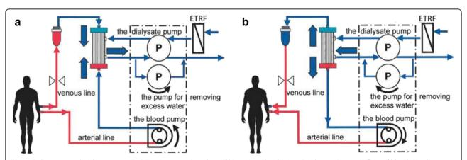
**Fig. 4** Fully automated dialysis system (FADS) **a** Automated guiding of blood into the dialyzer. *Red lines* indicate the flow of blood. *Blue lines* indicate the flow of the dialysate. *Thick blue arrows* indicate the direction of dialysate flow. **b** Blood return and collection. *Red lines* indicate the flow of blood, and *blue lines* indicate the flow of the dialysate. *Thick blue arrows* indicate the direction of the dialysate flow
